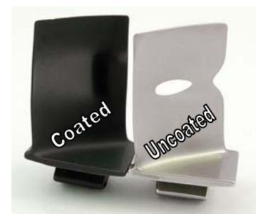
BlackGold™ after 3 kg of volcanic ash compared to uncoated at 2 kg
