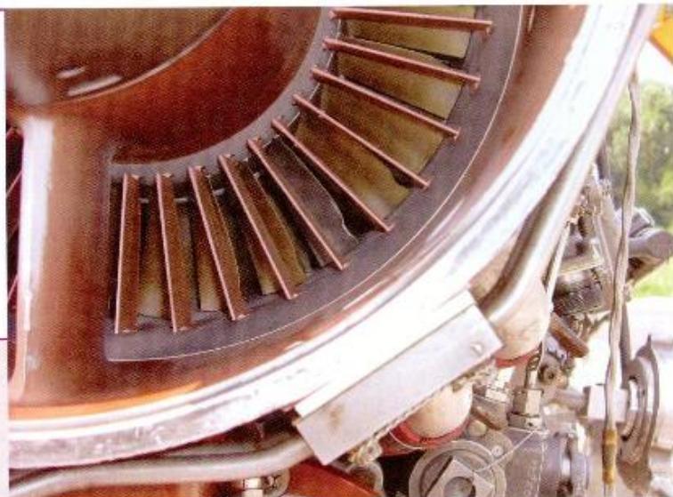
T58 compressor blades were coated with ER7 to prevent the leading edge curl and other damage encountered in sandy environments.
