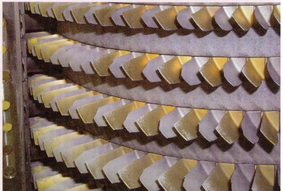
A T64 "rainbow" test engine shows erosive damage of sand ingestion tests on uncoated compressor blades.
